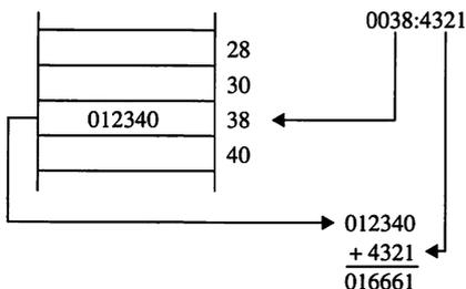
**Figure 2-4.** Decoding an 80286 protected-mode segmented address. The segment selector 38H indicates an entry in a segment descriptor table. The segment descriptor contains a 24-bit segment base address which is added to the offset 4321H to give the 24-bit physical address 016661H.
