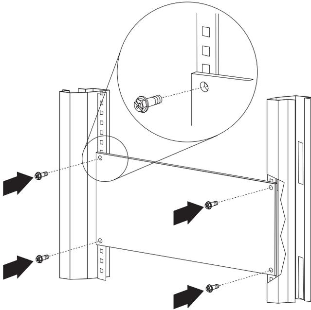
5. Tighten the four screws.
